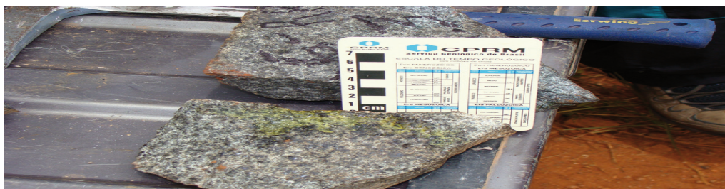
Figure 3. Samples of diabase from Taiano (municipality of Alto Alegre) with strong positive phosphomolybdate test.
